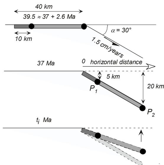
**Fig. 4** Model geometry, the PM segment goes up by simple shear.
